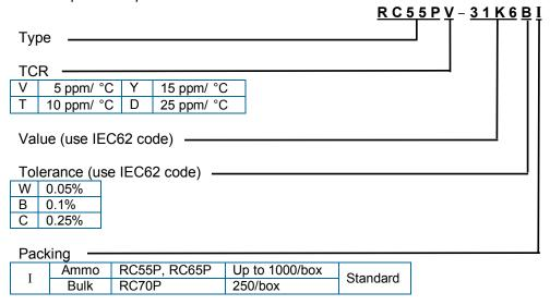
For 5ppm/°C screened product, replace the packing suffix with SC. Example: RC55PV-31K6BSC
